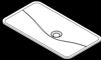
Built-in basin, rectangular, 700 x 385 mm, glazed inside and outside, for installation from above, without tap hole and overflow, includes chrome-plated drain valve and fixing set
