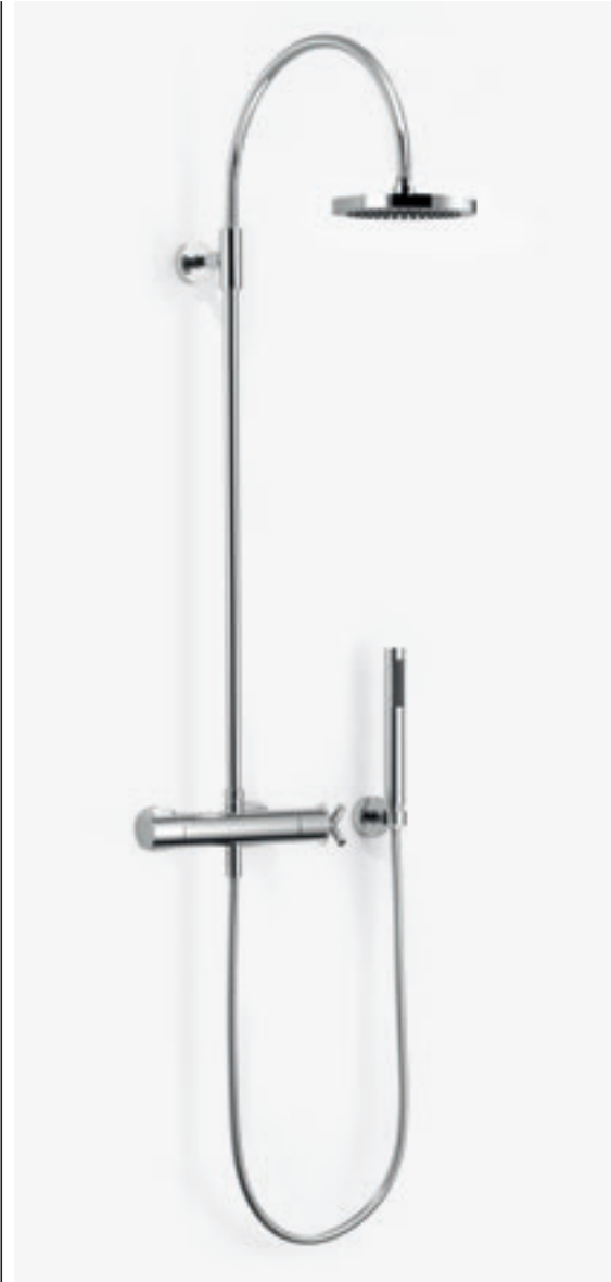
34 457 892 1/2" wall-mounted shower thermostat, Ø 220 mm Termostato doccia esterno 1/2", Ø 220 mm Termostato de ducha 1/2" para montaje a pared, Ø 220 mm [14 l/min.]
