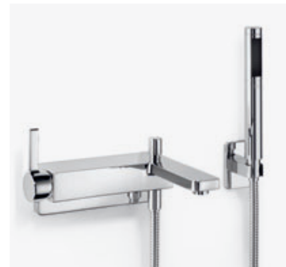
33 233 710 / 33 200 710 Wall-mounted single-lever bath mixer with/without shower set Miscelatore monocomando vasca esterno con/senza doccetta Monomando de ducha/bañera para montaje a pared con/sin ducha de mano [17 l/min.]
